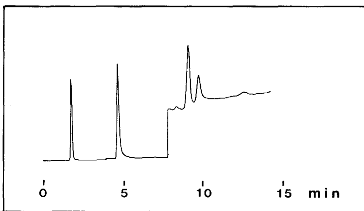
Fig. 6. Chromatogram from a working atmosphere containing N-methylmorpholine (1.75 min, 2600 \text{ ng}/\mu\text{l} ), DABCO (4.7 min, 22 \text{ ng}/\mu\text{l} ), 2,6-TDA (9.2 min, 1.2 \text{ ng}/\mu\text{l} ) and 2,4-TDA (9.9 min, 1.4 \text{ ng}/\mu\text{l} ). Injection volume: 1.6 \mu\text{l} . Attenuation: 2^8 \cdot 10^{-10}\text{--}2^{-4} \cdot 10^{-10} A f.s. Column temperature: 80 to 210^\circ\text{C} at 21^\circ\text{C}/\text{min} . Other parameters as in Fig. 1.
